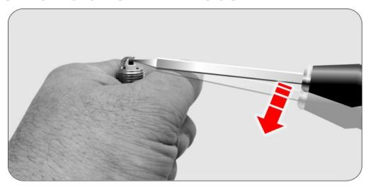
Using screwdriver (this operation requires a certain skill). Insert the scrwedriver between external and central electrode in the axle of external electrode the way the screwdriver touched only external electrode. Lever the external electrode by several tenths of milimetre over the back of thumb.
