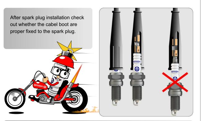
Spark plugs do not require any maintenance during the replacement interval. Certain level of maintenance is, however, required by the vehicle whose part the spark plugs are. All deficiencies caused by an insufficient vehicle maintenance can be reflected on the spark plug. That is why we recommend, within the framework of prevention, to check the spark plugs at least once a year. Their appearance reflects technical conditions of your vehicle.
